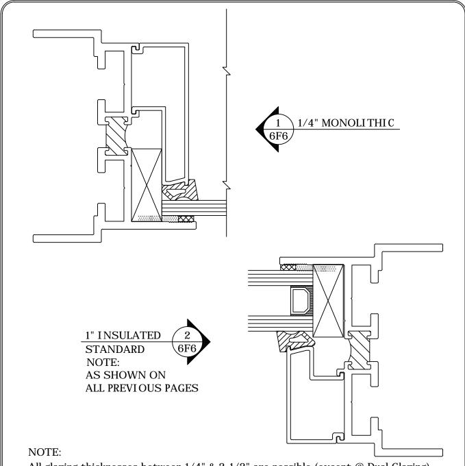
All glazing thicknesses between 1/4" & 2-1/2" are possible (except @ Dual Glazing). Win-Vent supplies setting blocks & neoprene gaskets. Glazing beads are factory notched around setting blocks where required. Glazing tape thickness is 1/8".
